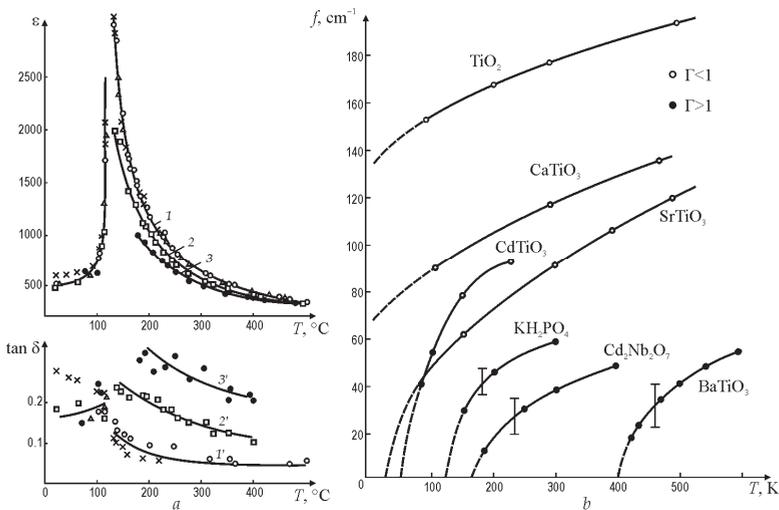
Fig.10. Paraelectrics at microwaves: BaTiO<sub>3</sub>  $\epsilon$  (1, 2, 3) and  $\text{tan}\delta$  (1', 2', 3') temperature dependence at different frequencies: 1 - 9.4-37 GHz; 2 - 46 GHz; 3 - 76 GHz (a); soft modes frequency dependence for various paraelectrics obtained by microwave and far infrared experiments (b)
