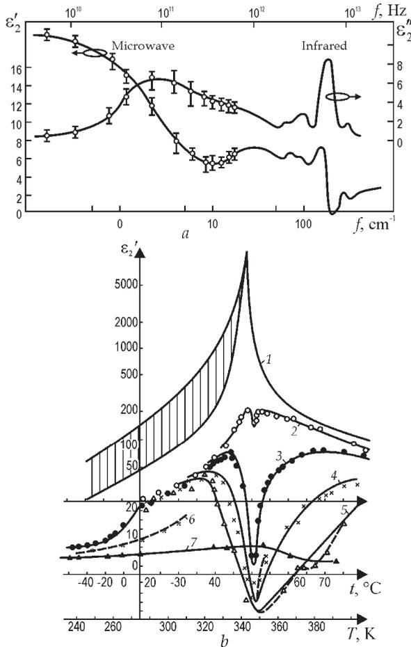
Fig. 6. TGS crystals microwave study:  $\epsilon'_2$  and  $\epsilon''_2$  frequency dependence at 300 K (*a*);  $\epsilon'_2$  temperature dependence at frequencies: 1 – 1 KHz, 2 – GHz, 3 – 16 GHz, 4 – 26 GHz, 5 – 37 GHz, 6 – 80 GHz, 7– 250 GHz (*b*)
