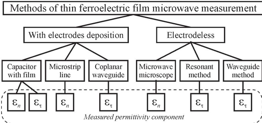
Fig. 12. Microwave methods for ferroelectric films study
