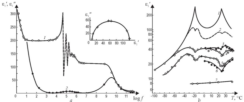
Fig. 5. Rochelle Salt microwave study:  $\epsilon'_1$  and  $\epsilon''_1$  frequency dependence at 18°C (a);  $\epsilon'_1$  temperature dependence at frequencies (in GHz): 1 - 0.8; 2 - 5.1; 3 - 8.4; 4 - 10.2; 5 - 20.5; 6 - 27; 7 - 250 (b)
