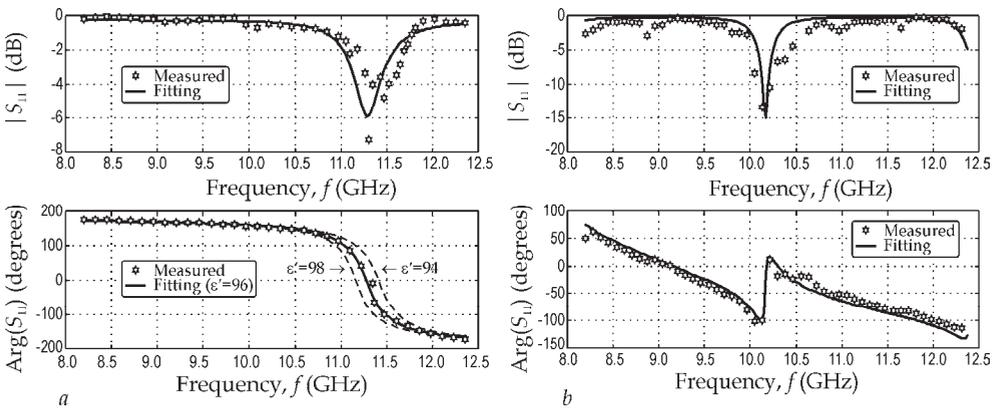
Fig. 3. Measured data and processing for reflection experiments: TiO<sub>2</sub>,  $\epsilon = 96$ , thickness 2.03 mm (a); SrTiO<sub>3</sub> of 3.89 mm thickness with 6.56 mm teflon transformer (b)
