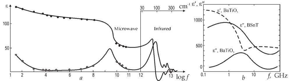
Fig. 9. Ferroelectric permittivity frequency dependence at 300 K: PbTiO<sub>3</sub> ceramics 1 - ε' and 2 - ε'' (a); ceramics BaTiO<sub>3</sub> and Ba(Ti,Sn)O<sub>3</sub> = BSnT microwave study (b)
