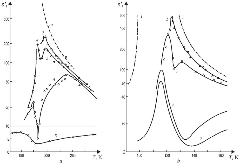
Fig. 7. Microwave dielectric dispersion in ferroelectrics of KDP type:  $\text{KD}_2\text{PO}_4$   $\epsilon'_3(T)$  at frequencies: 1 - 0.3 GHz; 2 - 8.6 GHz; 3 - 9.7 GHz; 4 - 26 GHz; 5 - 250 GHz (*a*);  $\text{KH}_2\text{PO}_4$   $\epsilon'_3(T)$  at frequencies: 1 - 1 kHz, 2 - 9.4 GHz; 3 - 80 GHz, 4 - 200 GHz; 5 - 340 GHz (*b*)
