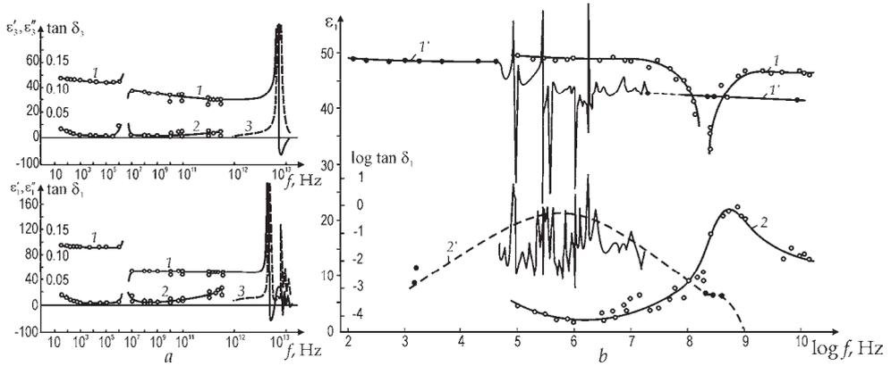
Fig. 8. Dielectric spectra of ferroelectric crystals at 300 K: single domain LiNbO<sub>3</sub> ε<sub>3</sub> and tanδ<sub>3</sub>, ε<sub>1</sub> and tanδ<sub>1</sub> (a); LiTaO<sub>3</sub>: 1 - ε<sub>1</sub>, 2 - tanδ<sub>1</sub> single domain; 1 - ε<sub>1</sub>, 2 - tanδ<sub>1</sub> for multidomain crystal (b)
