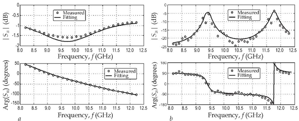
Fig. 4. Measured data and processing for: 1.51mm BaTiO<sub>3</sub> with 6.56 mm teflon transformer (a), reflection experiment; 3.89 mm SrTiO<sub>3</sub>, transmission experiment (b)
